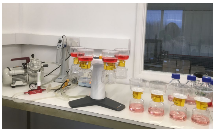
Figure 1: Experimental Setup for Filtration of Challenge Suspension
