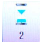
Test in progress. The hourglass "sand" will move to the bottom of the hourglass as the test progresses.
