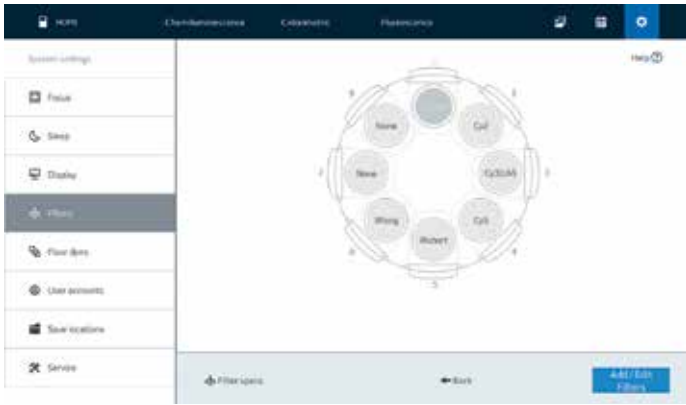
Fig 16. Follow the guided steps on the ImageQuant 800 software to easily set up custom filters or new LED-filter combinations for new dyes.
