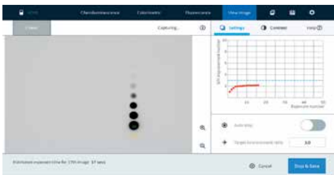
Fig 8. Observe how image quality improves in real time on the ImageQuant 800 system in SNOW exposure mode. The SNOW control window shows continuous image updates and the progression of signal-to-noise ratio improvement for your selected region of interest. The SNOW exposure mode can be set to stop automatically or by the user.
