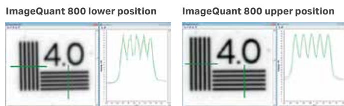
Fig 10. Epi-white imaging results in high-resolution images with excellent resolution. The four line-pair per mm pattern in a resolution test chart #2 (Applied Image, Inc.) shows clearly separated lines in both the lower and upper tray positions. The field of view in the upper position is 80 × 110 mm compared to 160 × 220 mm in the lower position.
